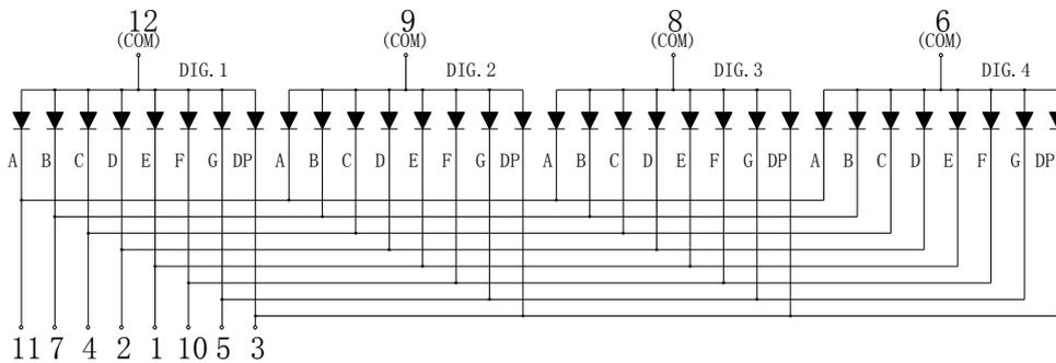
Internal Circuit Diagram (Common Cathode)
