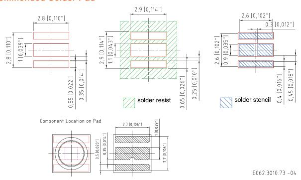
For superior solder joint connectivity results we recommend soldering under standard nitrogen atmosphere. In case the PCB layout of the application is intended to be used with other OSLON derivates or in future developed OSLON derivates, the heat sink must not be electrically connected to anode or cathode solder pad because of possible chip inverted polarity. Package not suitable for ultra sonic cleaning.
