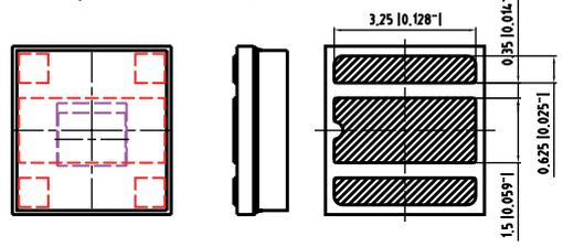
Alternative solder pad for exposed copper MCPCB - do not use exposed copper MCPCB for automotive applications.
