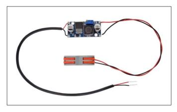
DC converter: In 9~36V, Out 5V 1A.
