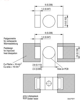
For superior solder joint connectivity results we recommend soldering under standard nitrogen atmosphere. Package not suitable for ultra sonic cleaning.
