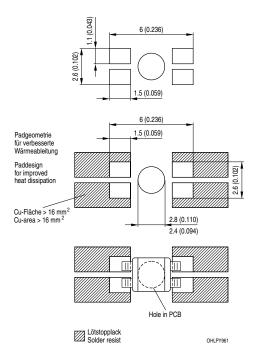
For superior solder joint connectivity results we recommend soldering under standard nitrogen atmosphere.
