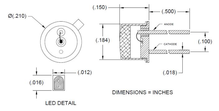
>Soldering Conditions: 260°C 1/16 inch away from case for 3 seconds max.
