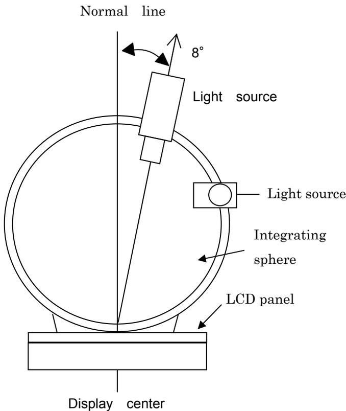
Figure 7-2 Contrast ratio, Reflection ratio, Panel chromaticity
