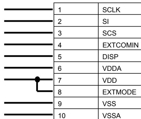
Figure 4-1 Recommended circuit
