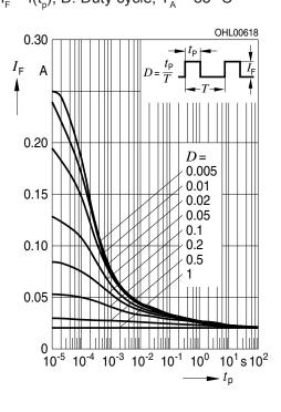
$I_{_{\rm F}} = f(t_{_{\rm D}})$ ; D: Duty cycle;  $T_{_{\rm A}} = 25 \text{ °C}$
