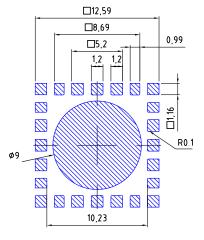
solder stencil recommended stencil thickness 200µm
