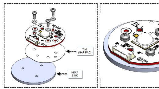
Mounting structure (exploded view)
