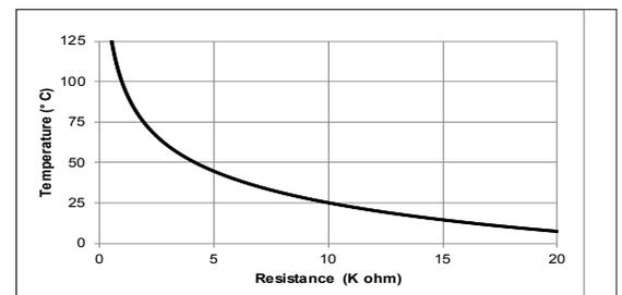
The thermistor used in CBT-120 devices mounted on coreboards is from Murata Manufacturing Co. The global part number is NCP18XH103J03RB. Please see <http://www.murata.com/> for details on calculating thermistor temperature.
