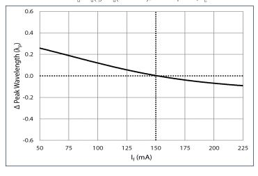
Temperature:  $\Delta \lambda_d = \lambda_d(T_c) - \lambda_d(25^{\circ}C)$ , 20 ms pulse,  $I_f = 150$  mA
