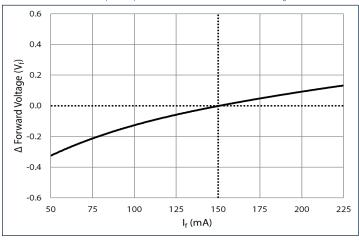
Temperature:  $\Delta V_f = V(T_c) - V(25^{\circ}C)$ , 20 ms pulse,  $I_f = 150$  mA
