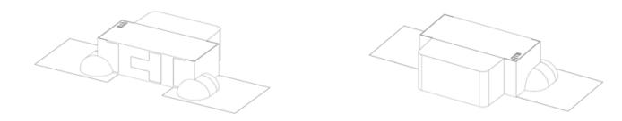
Note: The amount of solder paste applied as shown in the picture is just for illustration purpose only. When mounting and soldering the LEDs, avoid excess solder paste from overflowing onto or near the epoxy lens.
