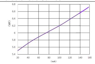
Forward Voltage vs. Forward Current
