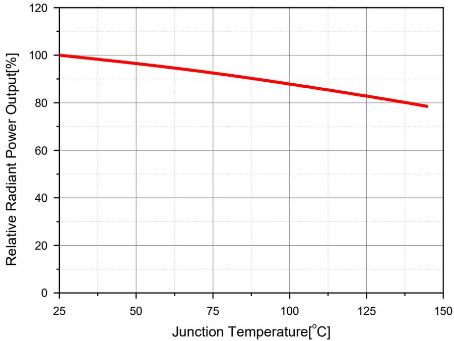
Relative Forward vs. Junction Temperature,  $I_F = 350\text{mA}$
