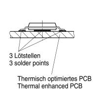
Lötstopplack Solder resist
