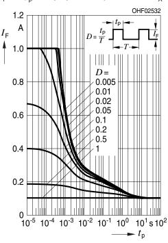
$I_{_{F}}$  = f (t<sub>p</sub>); duty cycle D = parameter;  $T_{_{A}}$  = 25°C
