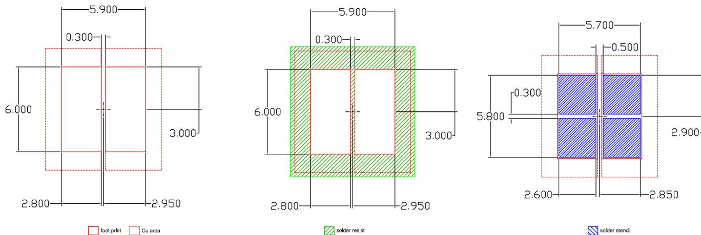
For superior solder joint connectivity results we recommend soldering under standard nitrogen atmosphere. Further information can be found in our Application Note: "Handling and Processing Details for Ceramic LEDs". Package not suitable for any kind of wet cleaning or ultrasonic cleaning.
