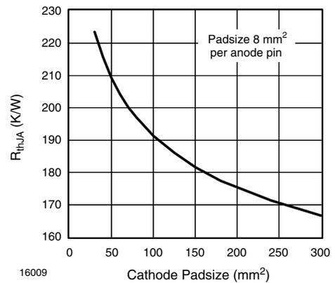
Fig. 5 - Thermal Resistance Junction Ambient vs. Cathode Padsizes
