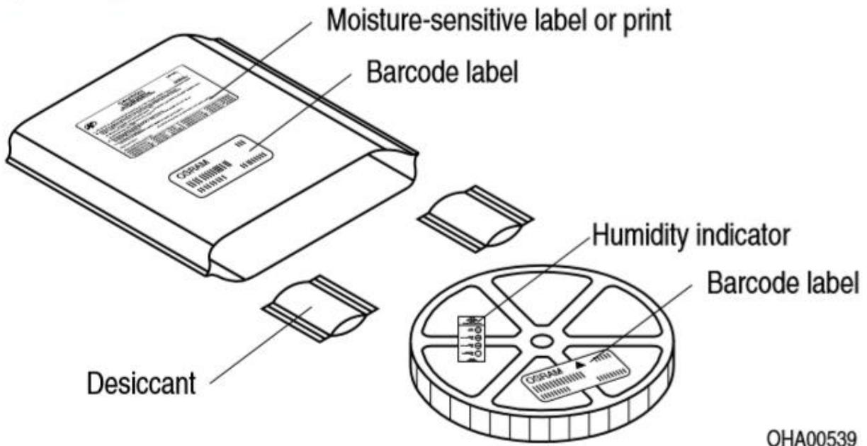
Moisture-sensitive product is packed in a dry bag containing desiccant and a humidity card according to JEDEC-STD-033.
