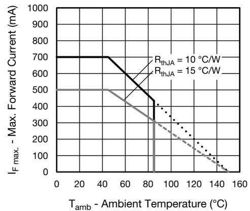
Fig. 5 - Maximum Forward Current vs. Ambient Temperature
