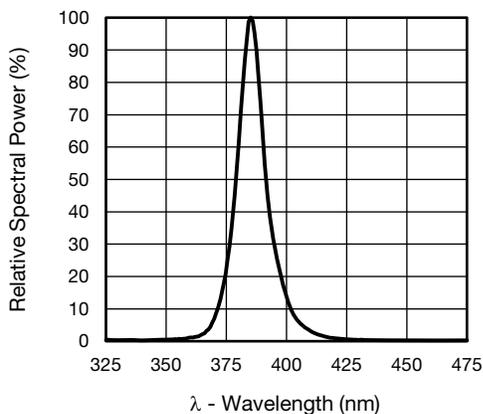
Fig. 3 - Relative Spectral Power vs. Wavelength
