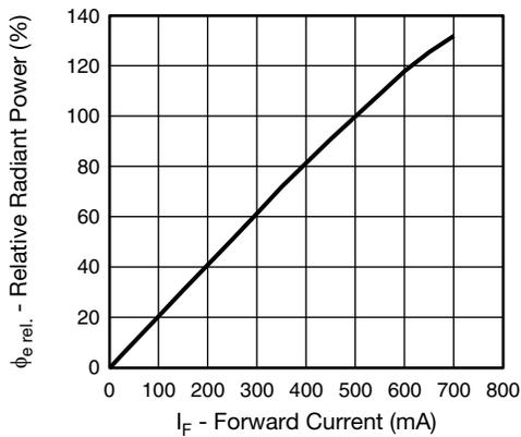
Fig. 1 - Relative Radiant Power vs. Forward Current
