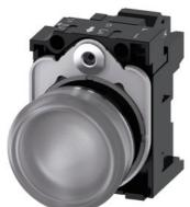
Indicator lights, 22 mm, round, metal, shiny, clear, lens, smooth, with holder, LED module with integrated LED 24 V AC/DC, spring-type terminal, with laser labeling, lower case
