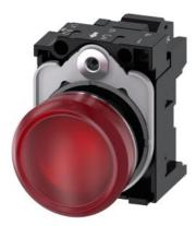
Indicator lights, 22 mm, round, metal, shiny, red, lens, smooth, with holder, LED module with integrated LED 24 V AC/DC, spring-type terminal, with laser labeling, lower case
