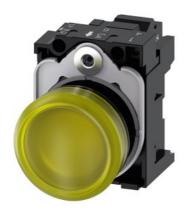
Indicator light, 22 mm, round, plastic, yellow, lens, smooth, with holder, LED module, with integrated LED 24 V AC/DC, spring-type terminal, with laser labeling, upper case and lower case, always upper case at beginning of line
