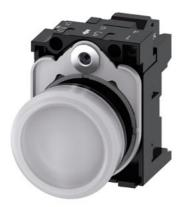
Indicator lights, 22 mm, round, plastic, white, lens, smooth, with holder, LED module, with integrated LED 24 V AC/DC, Spring-type terminal
