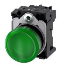
Indicator lights, 22 mm, round, plastic, green, lens, smooth, with holder, LED module, with integrated LED 24 V AC/DC, screw terminal, with laser labeling, upper case
