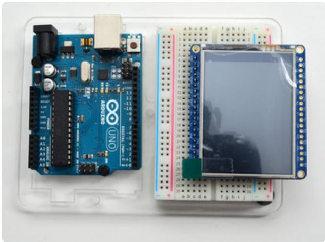
If your display isn't taped down to the breakout PCB, peel off the tape covering and press down so the TFT sticks to the circuit board
