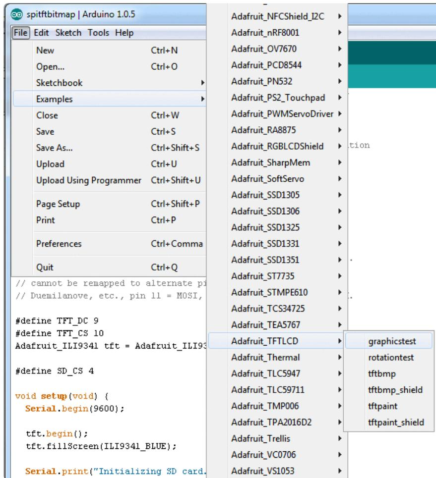
After restarting the Arduino software, you should see a new **example** folder called **Adafruit\_TFTLCD** and inside, an example called **graphicstest**. Upload that sketch to your Arduino. You may need to press the Reset button to reset the arduino and TFT. You should see a collection of graphical tests draw out on the TFT.
