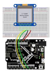
Microcontroller GND to LCD Gnd Microcontroller 5V to LCD Vin Microcontroller D13 to LCD Clk Microcontroller D11 to LCD DI Microcontroller D10 to LCD CS
