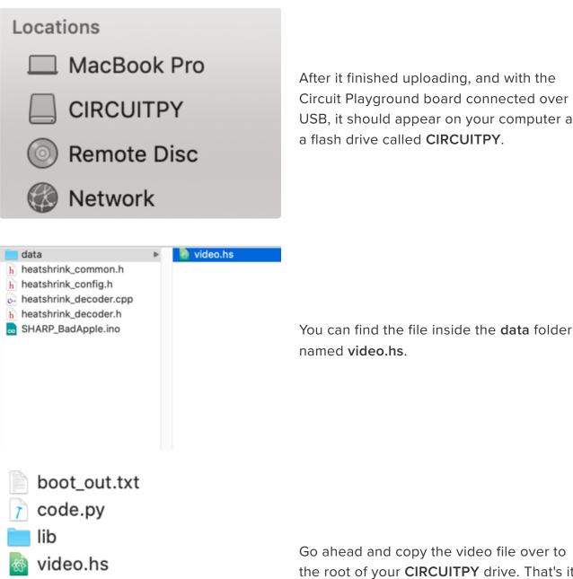
After it finished uploading, and with the Circuit Playground board connected over USB, it should appear on your computer as a flash drive called CIRCUITPY.
