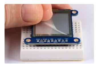
Remove the Protective Film After soldering is complete. Gently peel the film from the display.
