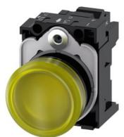
Indicator lights, 22 mm, round, plastic, yellow, lens, smooth, with holder, LED module with integrated LED 110 V AC, spring-type terminal, with laser labeling, symbol number according to, ISO 7000 or IEC 60417
