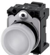
Indicator lights, 22 mm, round, metal, shiny, white, lens, smooth, with holder, LED module with integrated LED 230 V AC, Spring-type terminal
