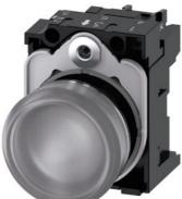
Indicator lights, 22 mm, round, Metal, shiny, clear, lens, smooth, with holder, LED module with integrated LED 230 V AC, screw terminal, with laser labeling, lower case
