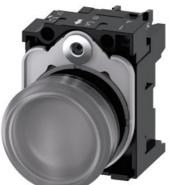
Indicator lights, 22 mm, round, plastic, clear, lens, smooth, with holder, LED module, with integrated LED 24 V AC/DC, screw terminal, with laser labeling, inscription or symbol Customer-specific selection with SIRIUS ACT configurator (CIN)
