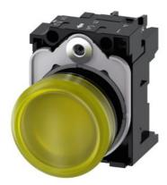
Indicator lights, 22 mm, round, plastic, yellow, lens, smooth, with holder, LED module, with integrated LED 24 V AC/DC, screw terminal, with laser labeling, inscription or symbol Customer-specific selection with SIRIUS ACT configurator (CIN)
