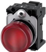
Indicator light, 22 mm, round, metal, shiny, red, lens, smooth, with holder, LED module with integrated LED 24 V AC/DC, spring-type terminal, with laser labeling, upper case and lower case, always upper case at beginning of line
