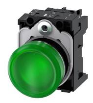
Indicator lights, 22 mm, round, metal, shiny, green, lens, smooth, with holder, LED module with integrated LED 110 V AC, screw terminal, with laser labeling, symbol number according to, ISO 7000 or IEC 60417
