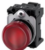
Indicator lights, 22 mm, round, Metal, shiny, red, lens, smooth, with holder, LED module with integrated LED 230 V AC, spring-type terminal, with laser labeling, upper case
