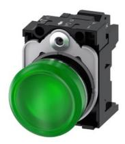
Indicator lights, 22 mm, round, Metal, shiny, green, lens, smooth, with holder, LED module with integrated LED 230 V AC, spring-type terminal, with laser labeling, inscription or symbol Customer-specific selection with SIRIUS ACT configurator (CIN)
