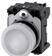
Indicator lights, 22 mm, round, metal, shiny, white, lens, smooth, with holder, LED module with integrated LED 110 V AC, screw terminal, with laser labeling, inscription or symbol Customer-specific selection with SIRIUS ACT configurator (CIN)
