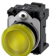
Indicator lights, 22 mm, round, metal, shiny, yellow, lens, smooth, with holder, LED module with integrated LED 230 V AC, spring-type terminal, Z=20-unit packaging
