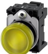
Indicator lights, 22 mm, round, metal, shiny, yellow, lens, smooth, with holder, LED module with integrated LED 110 V AC, spring-type terminal, with laser labeling, upper case
