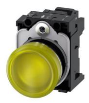
Indicator lights, 22 mm, round, metal, shiny, yellow, lens, smooth, with holder, LED module with integrated LED 24 V AC/DC, spring-type terminal, with laser labeling, upper case and lower case, always upper case at the beginning of the word
