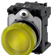
Indicator lights, 22 mm, round, metal, shiny, yellow, lens, smooth, with holder, LED module with integrated LED 24 V AC/DC, screw terminal
