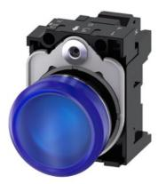
Indicator lights, 22 mm, round, metal, shiny, blue, lens, smooth, with holder, LED module with integrated LED 110 V AC, spring-type terminal, with laser labeling, inscription or symbol Customer-specific selection with SIRIUS ACT configurator (CIN)
