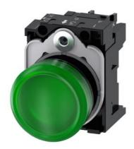
Indicator lights, 22 mm, round, plastic, green, lens, smooth, with holder, LED module, with integrated LED 24 V AC/DC, screw terminal, with laser labeling, symbol number according to, ISO 7000 or IEC 60417
