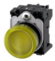
Indicator lights, 22 mm, round, plastic, yellow, lens, smooth, with holder, LED module with integrated LED 110 V AC, screw terminal, with laser labeling, upper case
