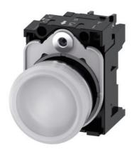
Indicator lights, 22 mm, round, metal, shiny, white, lens, smooth, with holder, LED module with integrated LED 110 V AC, screw terminal, with laser labeling, upper case
