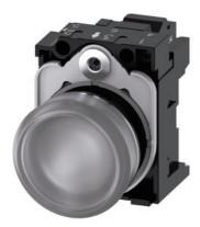
Indicator lights, 22 mm, round, Metal, shiny, clear, lens, smooth, with holder, LED module with integrated LED 230 V AC, spring-type terminal, with laser labeling, symbol number according to, ISO 7000 or IEC 60417
