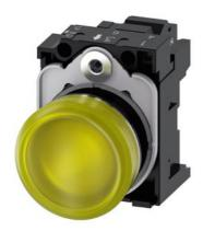
Indicator lights, 22 mm, round, metal, shiny, yellow, lens, smooth, with holder, LED module with integrated LED 24 V AC/DC, spring-type terminal, with laser labeling, symbol number according to, ISO 7000 or IEC 60417
