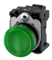
Indicator lights, 22 mm, round, plastic, green, lens, smooth, with holder, LED module, with integrated LED 24 V AC/DC, spring-type terminal, with laser labeling, upper case
